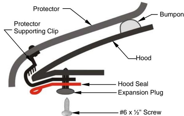
8. Working from left to right insert the brackets in between the hood and the hood seal. Then, using the same left to right technique, push the brackets over the edge of the hood. Make sure the protector is centered on the hood; make sure the brackets are fully seated against the hood edge.
