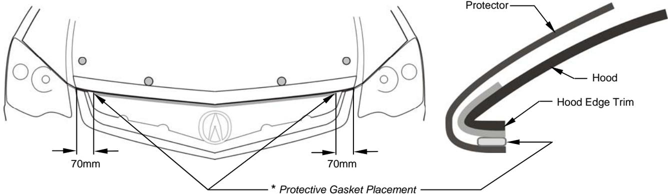
6. Center the protector on the hood by aligning the two (2) indents in the leading edge of the protector with the two (2) square cutouts on the underside of the hood.
