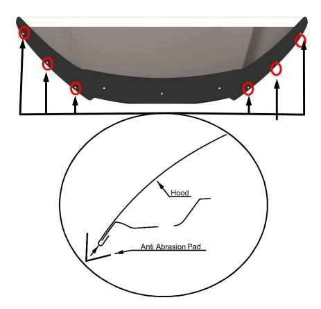
8. Peel and fold the anti-abrasion pads in half over the edge of the hood in line with the three holes in the protector over each of the headlights. *See Illustration*. Repeat for remaining push-type retainers.
