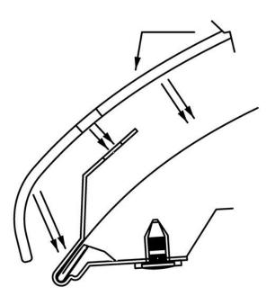
6. Place the hood protector on the hood, resting on the three metal brackets.
