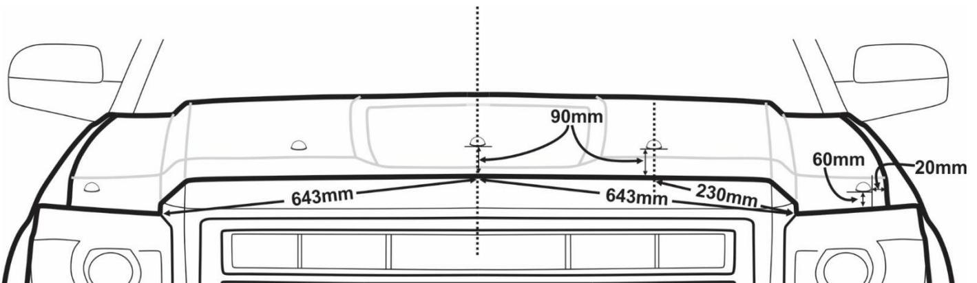
3. Clean the area indicated in the illustration to a point approximately 24" on each side of the center of the hood.
