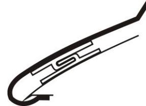
5. Raise the hood of the vehicle without disturbing the hood deflector placement. Insert the expansion plugs through the holes in the deflector and into the holes in the hood. Be sure that the deflector is well seated against the hood, then insert and tighten the screws into the expansion plugs.
