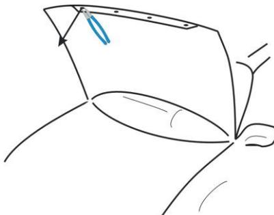
3. Attach the pedestals clips from the kit to the clips already attached to the deflector. See below.
