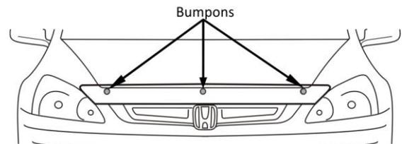
7. On some vehicles it may be necessary to adjust the hood bumpers and/or latch for proper clearance
