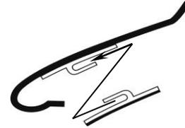
4. Peel the protective backing from the tape on the pedestals. While keeping the pedestals away from the hood surface, nest the tab of the deflector under the hood, center it on the hood, rotate and press the deflector into place. Push down the pedestals clips to make sure they are properly adhered to the hood.
