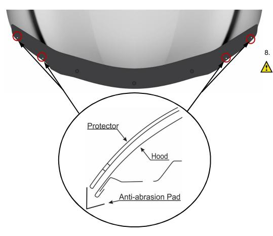
Peel and fold the remaining 4 antiabrasion pads in half over the edge of the hood in line with the two holes in the protector over each of the headlights. See Illustration.
