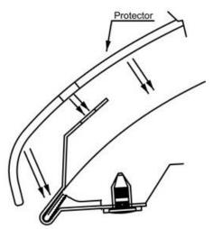
6. Place the hood protector on the hood, resting on the four metal brackets.
