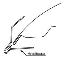
Install the three metal brackets on the hood edge over the anti-abrasion pads. Align the hole in the bottom leg of the bracket with the round hole in the hood. See Illustration.
