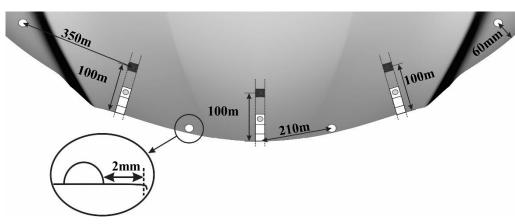
Install the three (3) black Bumpons behind the metal brackets and then the four (4) round Bumpons as shown. <u>Attention: Bumpons must be</u> <u>installed on the hood, not on the</u> <u>deflector!!!</u>
