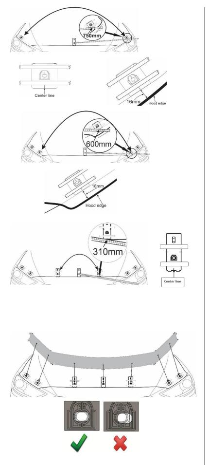
5. Dry fit the remaining pedestals using tape strips supplied or masking tape to temporarily hold them in position.
