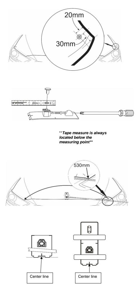
Install the two (2) bumpons as shown. <u>Attention: Bumpons must be installed</u> <u>on the hood, not on the protector!!!</u> If the bumpons are installed on the protector, they may wear through the paint.
