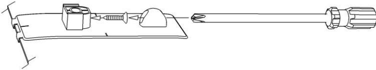
9. Start a #6 x 5/8 flat head screw into each pedestal a few turns. The tip of the screw must not protrude into the hole where the attachment pin will install later.
