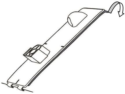
8. Remove the protective backing film from each of the adhesive pedestals and install them on the hood surface.
