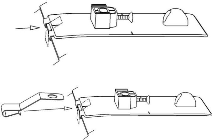
11. Push a metal mounting bracket over the hood edge on top of the anti abrasion pad installed previously. Ensure the bracket is fully engaged over the hood edge and the hole in the bracket is aligned with the hole in each of the pedestals.
