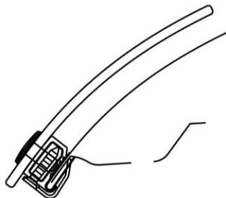
14. Peel and fold two (2) of the large anti-abrasion film pads in half over the hood edge aligned with the inner holes of the deflector in the area above the headlights.
