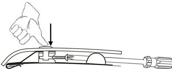
13. Maintain slight pressure on the pin, to ensure proper seating of the components, while simultaneously tightening the screw. Repeat for remaining pedestal locations.
