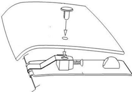
12. Place the deflector on the pedestals and drop a pin through the deflector and into the pedestal.
