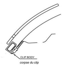
4. At the center, place a clip body over the anti-abrasion film pad on the edge of the hood.
