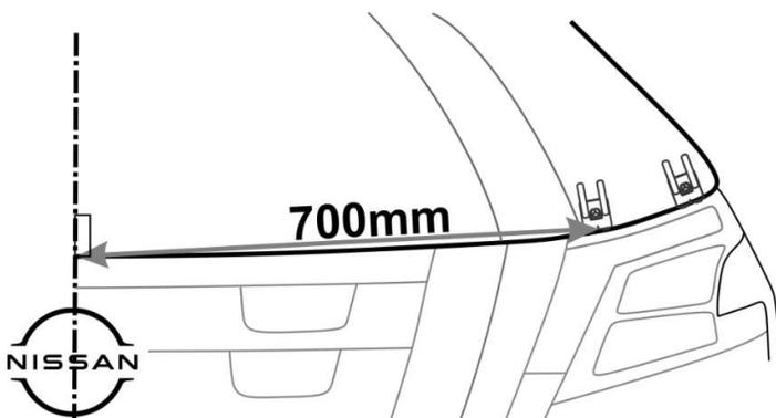
1. Use the Centre hole on the underside of the hood to reference the centre. Wrap an anti-abrasion film pad over the hood edge and put a mark on the antiabrasion pad where the centre is.
