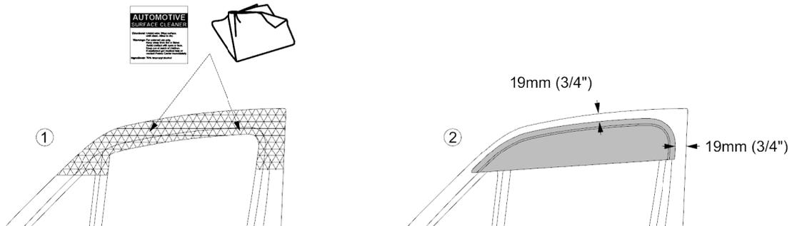
3. Starting at the back edge of one deflector, peel the first 5cm (2 inches) of the protective backing from the adhesive on the horizontal flange of the deflector. Peel the first 5cm (2 inches) of the protective backing from the vertical flange as well. Fold back the protective backing from the adhesive as shown in the illustration.
