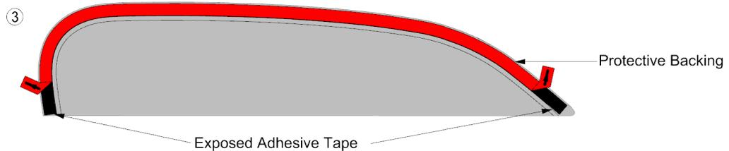
4. Reposition the deflectors to the door frames 19mm (3/4") from the edge of the door. If needed adjust the deflector for best fit.
