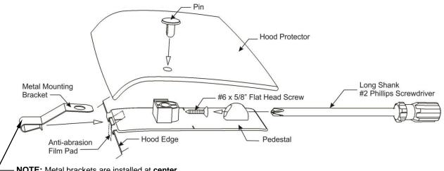
**NOTE:** Metal brackets are installed at **center** and **outside** locations **ONLY**.
