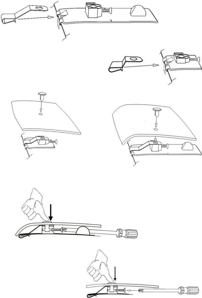
11. Push metal mounting brackets over the hood edge aligned with the anti-abrasion pads installed previously. Ensure each bracket is fully engaged over the hood edge and the hole in the bracket is aligned with the hole in the pedestal.
