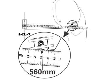
1. Position and hold the installation tape measure at the outside edge of the hood, at the dimension shown in the illustration.
