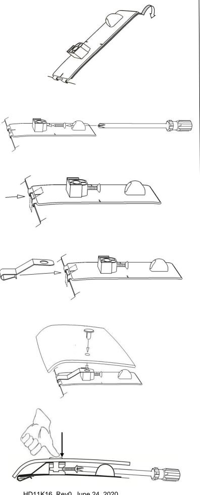
Remove the protective backing film from each of the adhesive pedestals and install them on the hood surface.
