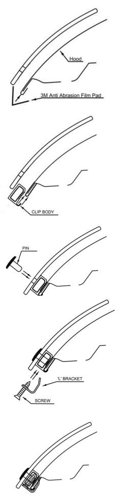
15. Peel and fold the four (4) large anti-abrasion film pads in half over the hood edge aligned with the outer holes of the deflector in the area above the headlights.
