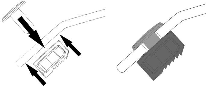
7. Place a pin through each of the (4) middle holes in the hood deflector and into the clip bodies as shown.
