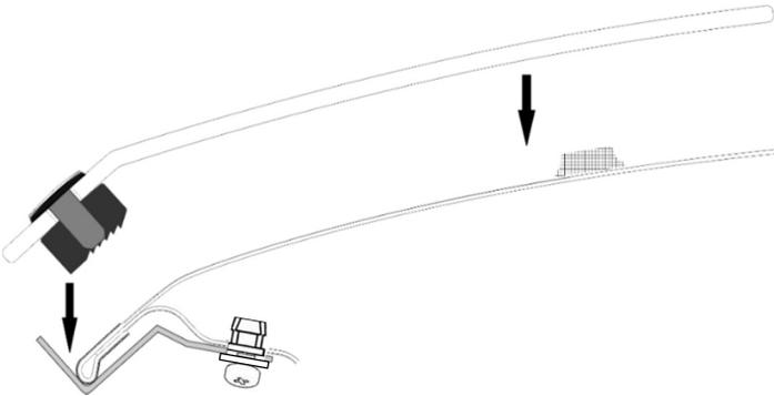
9. Insert a #6 x 5/8" flat head screw through each of the (4) metal mounting brackets and into the clip bodies.
