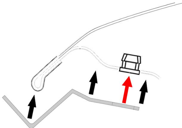
5. Position the metal mounting brackets over the hood edge (at the same (4) locations from the previous step) by aligning the hole in the bottom of the metal mounting bracket with the round hole in the square expansion plug.
