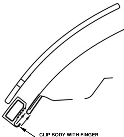
12. Place the clip bodies with fingers over each of the (4) anti-abrasion film pads on the edge of the hood.
