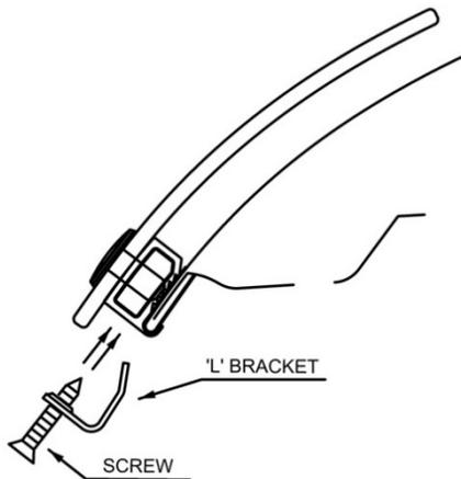
14. Insert #6 x 5/8" flat head screw through a "L" bracket and into each of the (4) clip bodies with fingers
