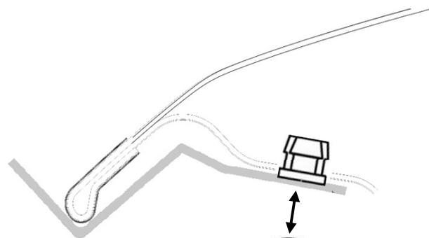
6. Secure the (4) metal mounting brackets by inserting the #10 x 5/8" pan head screw through the rubber bonded washer and into the square expansion plug.
