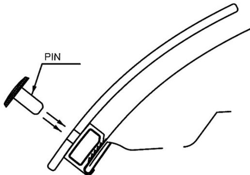
13. Insert a pin through the hood deflector into each of the (4) clip bodies with fingers.
