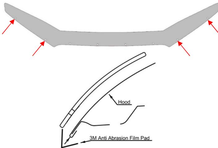
11. Peel and fold the remaining (4) anti-abrasion film pads in half over the hood edge aligned with the (4) outer holes in the hood deflector above the headlamps.
