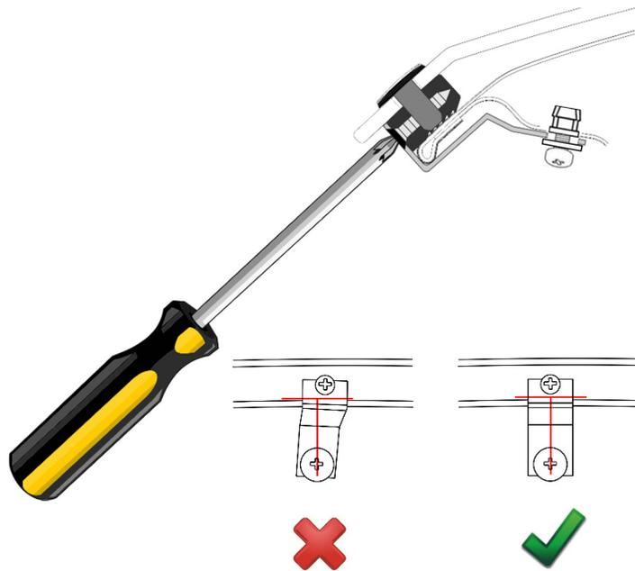
10. Ensure all (4) metal mounting brackets and clip bodies are properly aligned and tighten the screws.
