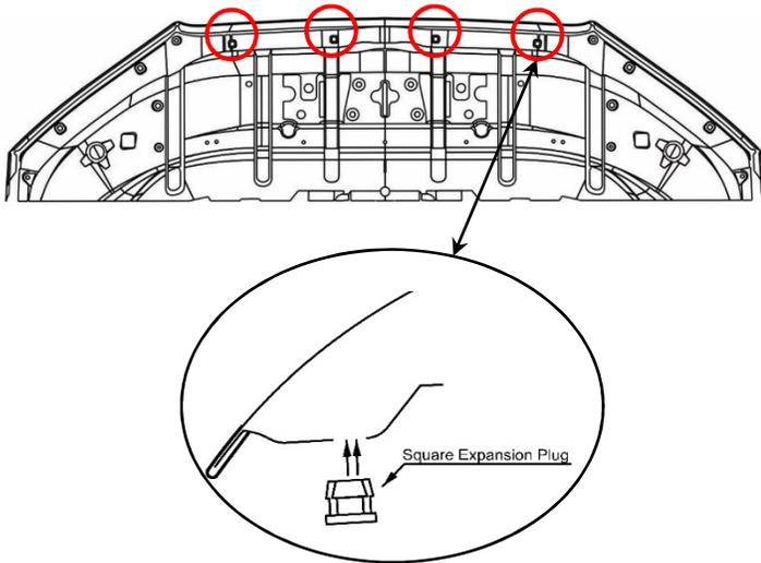
4. Insert square expansion plugs into the (4) holes in the hood inner as shown.
