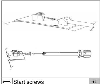
Start a screw into each pedestal a few turns. The tip of the screw must not protrude into the hole where the attachment pin will install later.
