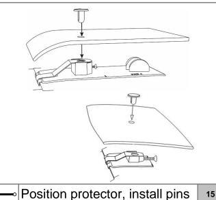
Place the protector on the pedestals and starting at the center position, install a pin through the protector and into the pedestal.
