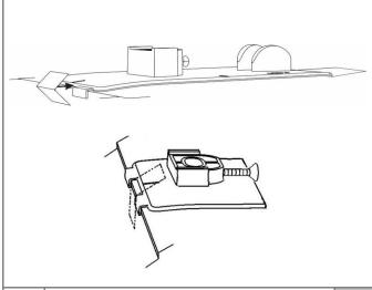
Peel and fold the anti-abrasion film pads in half over the hood edge between the fingers on each of the mounting pedestals.
