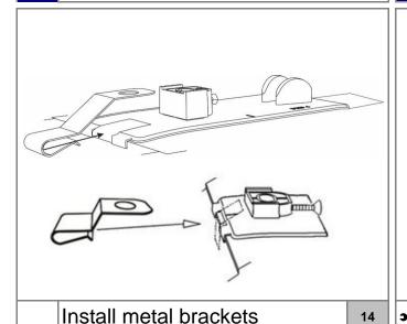
Push metal mounting brackets over the hood edge aligned with the anti-abrasion pads. Ensure the bracket is fully seated over the hood edge and the hole in the bracket is aligned with the hole in the pedestal.
