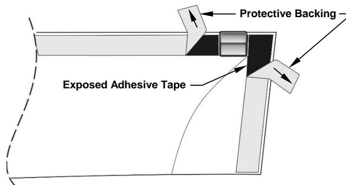
6. Reposition the visor on the window frame as described in steps #2 and #3. Adjust the visor for best fit. While pressing the visor into place, pull the protective backing out from between the visor and door frame without disturbing the fit of the visor.
