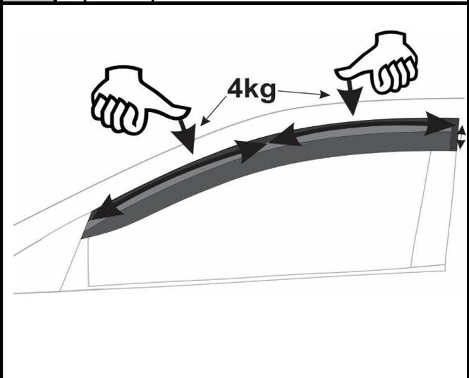
**6 "Wet out" adhesive tape with 4kg of force / Mouiller le ruban adhésif**
