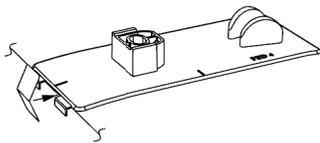
12. Peel and fold the anti-abrasion film pads in half over the hood edge between the fingers on each of the large pedestals in the locations shown.
