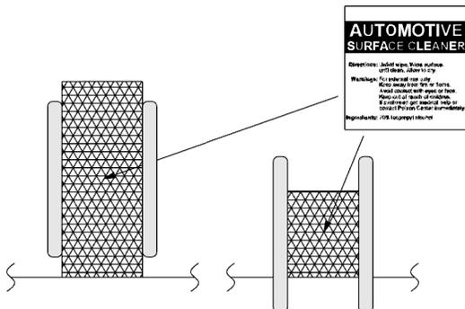
6. Dry fit the pedestals using tape strips supplied or masking tape to temporarily hold them in position. The positions of the pedestals are shown in the illustrations. Use the center line on the leading edge of the pedestals for accurate measuring. The pedestals install perpendicular to the hood edge.
