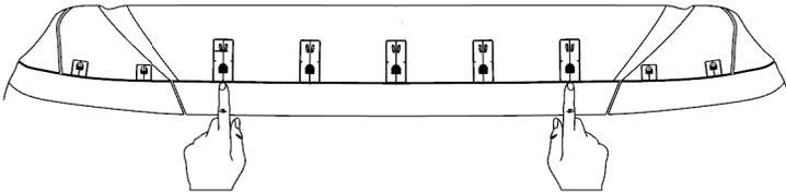
13. Push metal mounting brackets over the hood edge aligned with the anti-abrasion pads. Ensure the bracket is fully seated over the hood edge and the hole in the bracket is aligned with the hole in the pedestal.
