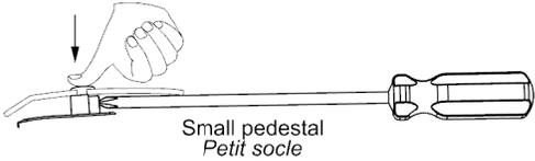
14. Place the hood protector on to the pedestals. Starting at the center and working outwards install the pins.
