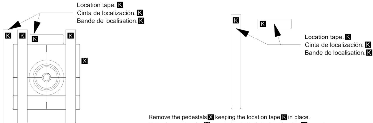
Remove the pedestals **X** keeping the location tape **K** in place.
