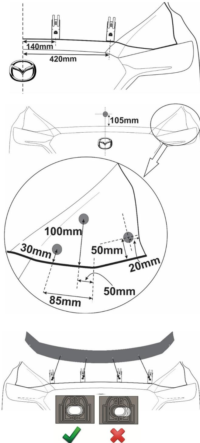
1. Locate the "How to find the centerline of the hood" supplement and, following the instructions, mark the center of the hood.
