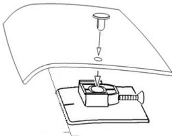
14. Start a screw into each pedestal a few turns. The tip of the screw must not protrude into the hole where the attachment pin will later install.
