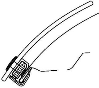
7. Ensure all the components are well seated together. Do a final check to ensure the protector is centered on the hood, and then tighten the screws into the clip bodies.
