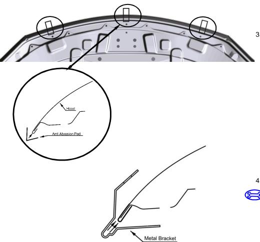
Open the hood of the vehicle. Peel and fold the anti-abrasion pads in half over the edge of the hood, in line with the 3(three) holes under the hood, as shown. See illustration.
