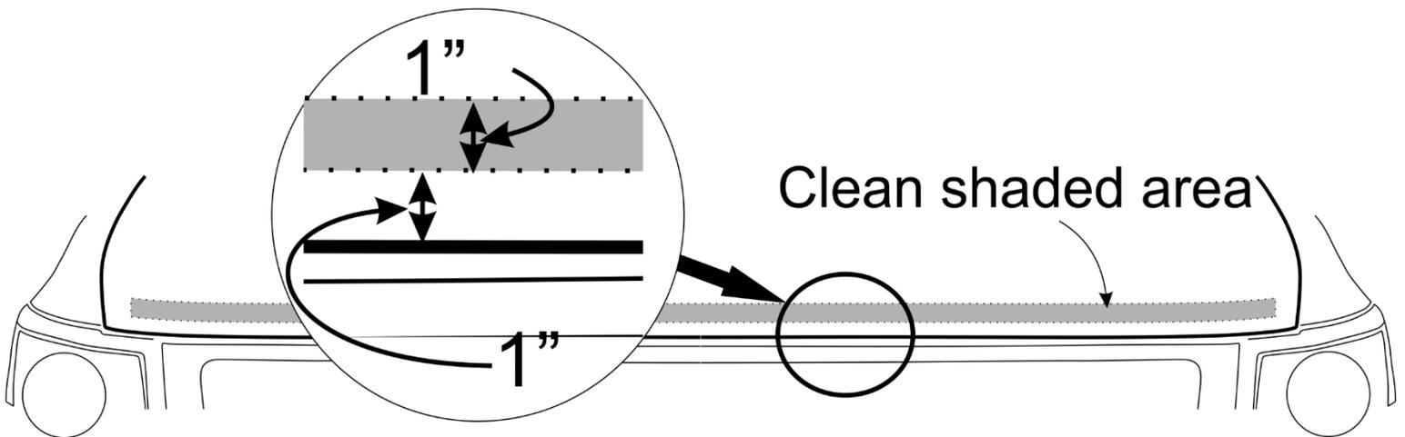
4. Center the "D" gasket laterally on the hood. 48" is provided. It may be necessary to trim the length slightly to fit the contours of the hood.
