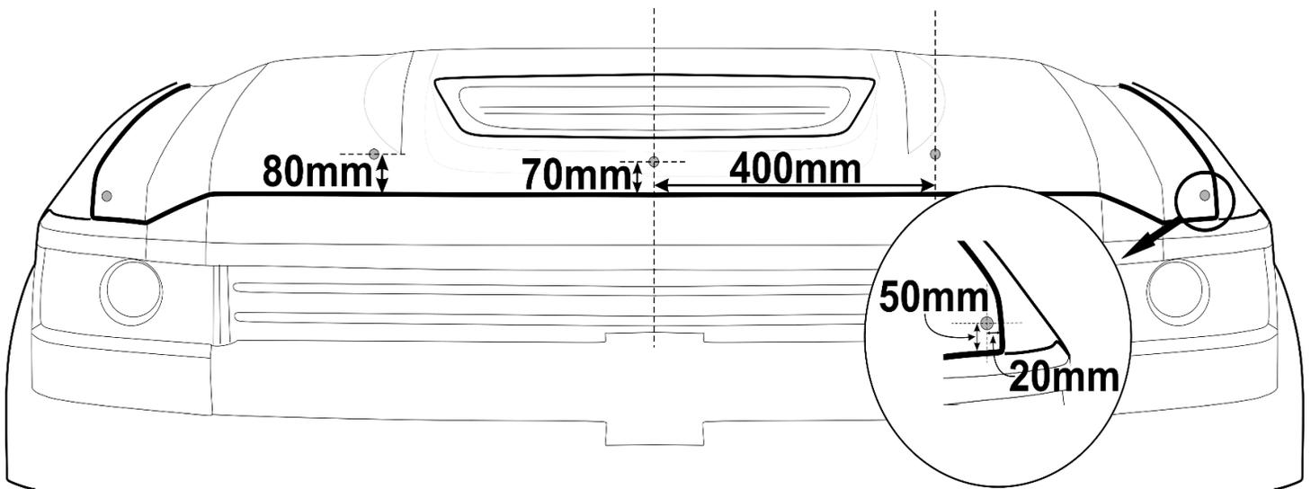
2. Clean the area indicated in the illustration to a point approximately 24" on each side of the center of the hood.
