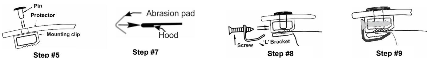
**NOTE: Do not pull on the protector when opening or closing the hood.**
