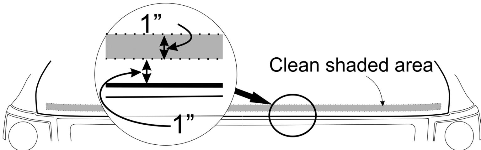
3. Center the "D" gasket laterally on the hood. 48" is provided. It may be necessary to trim the length slightly to fit the contours of the hood.
