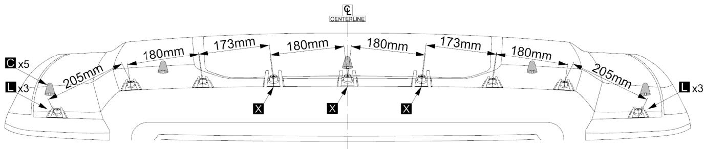
7 Place the hood protector **A** on the bumpers **C** make sure it is properly centered. Looking through holes, make sure each pedestal **L / X** is aligned with the hole in the protector.
