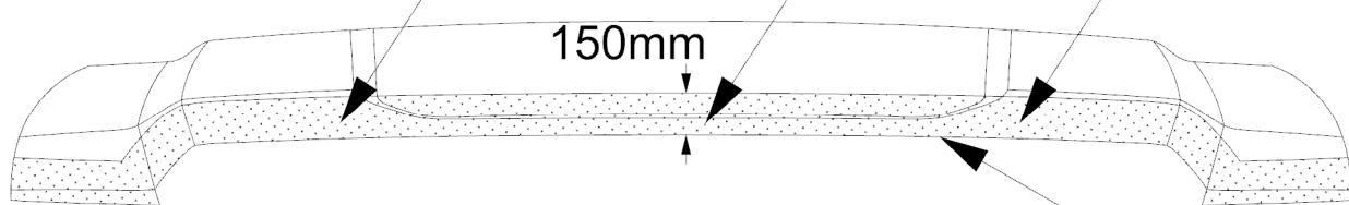
Using one of the surface wipes **B** provided and clean the first 150mm of front of the hood.
