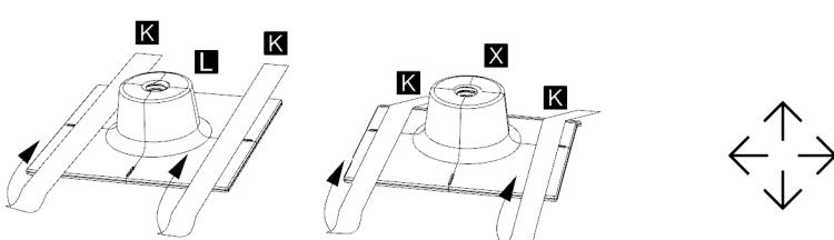
Remember the direction of adjustment, remove all tape. **K**
