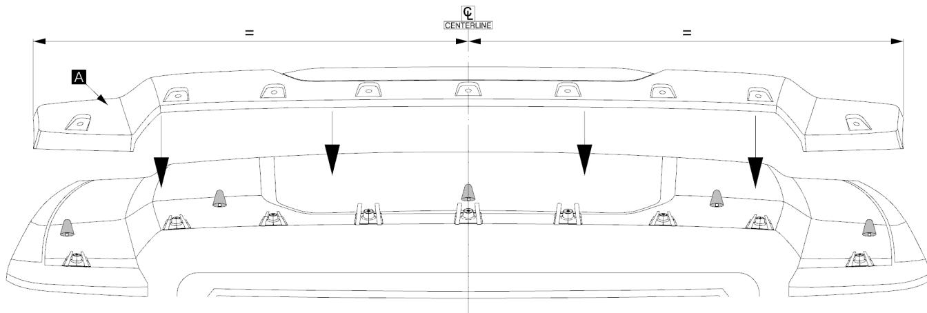
8 Pedestal **L / X** is aligned correctly.
