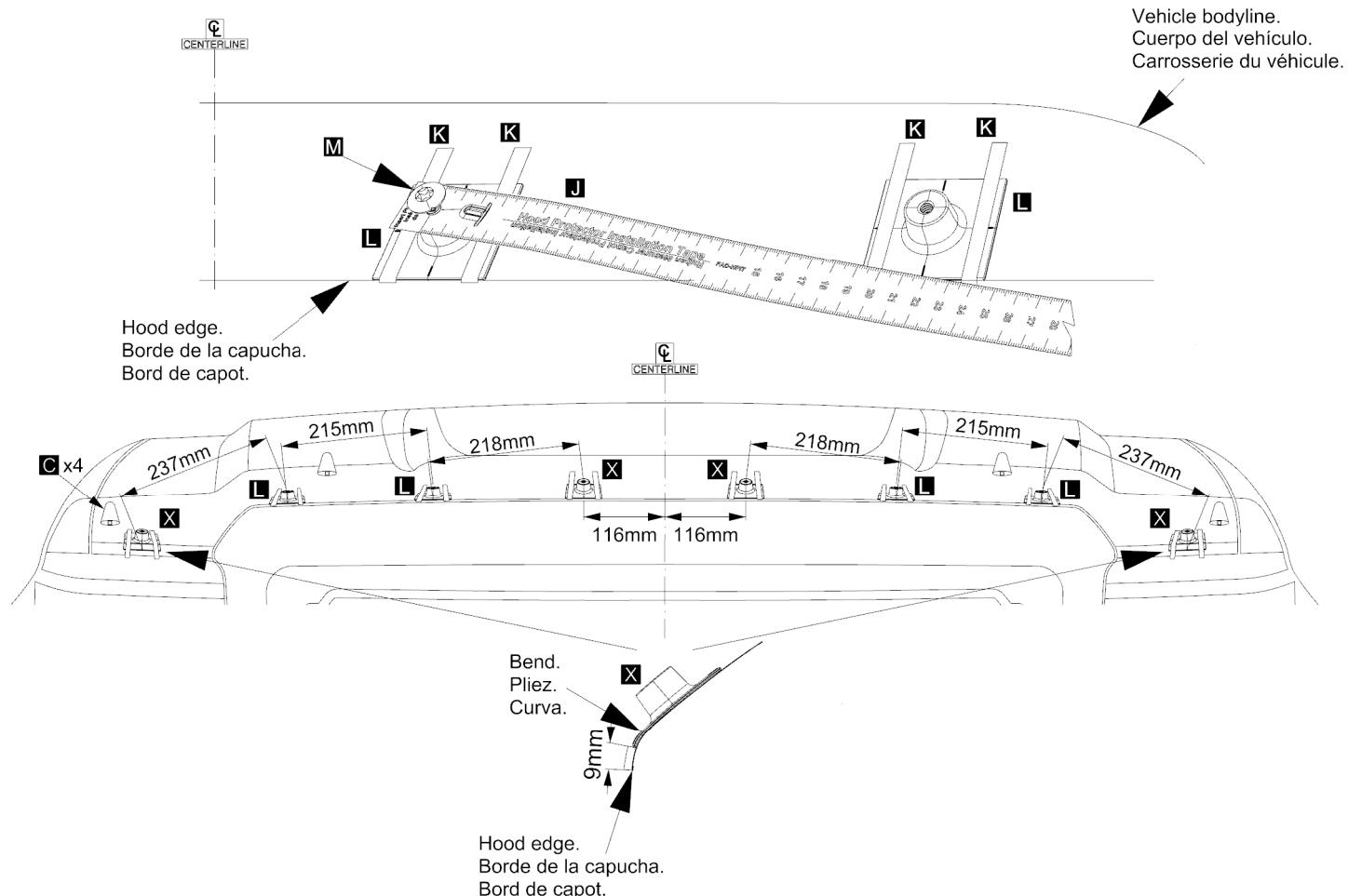
7 Place the hood protector **A** on the bumpers **C** make sure it is properly centered. Looking through holes, make sure each pedestal **X / L** is aligned with the hole in the protector.
