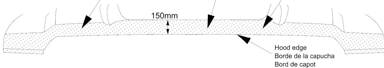
Using one of the surface wipes **B** provided and clean the first 150mm of front of the hood.
