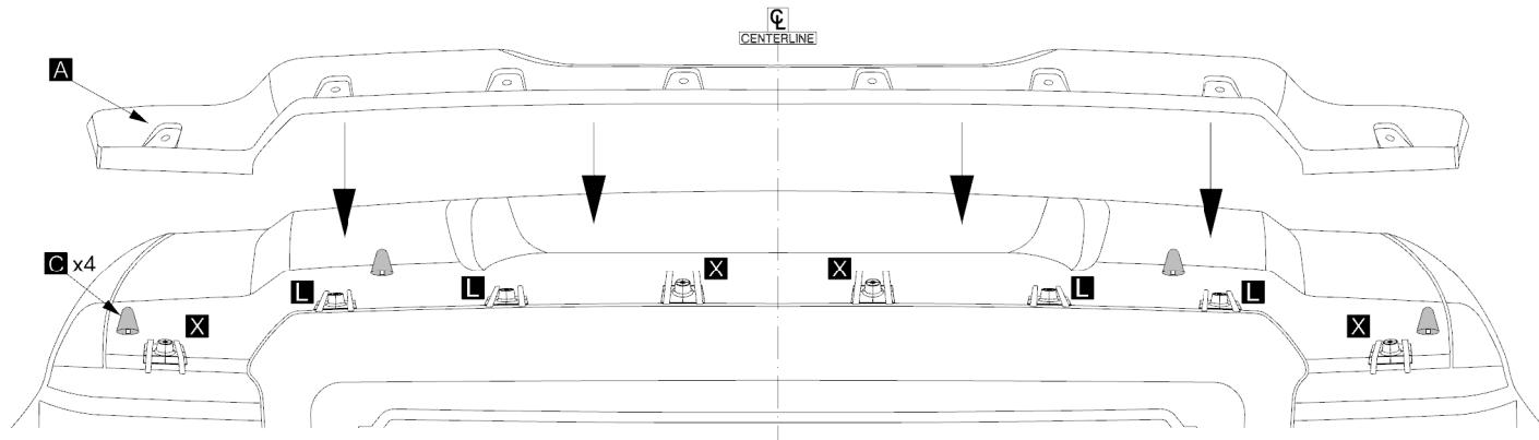
8 Pedestal **L / X** is aligned correctly.
