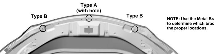
**NOTE: Use the Metal Bracket Guide** to determine which brackets go in
