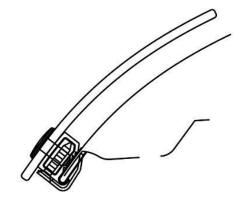
13. Make sure all the components are well seated together; the protector is centered on the hood, and, starting at the innermost clip locations, finish tightening the screws into the clips. *Do not overtighten.*
