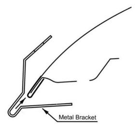
3. Install the (3) metal brackets on the hood edge over the anti-abrasion pads. Align the hole in the bottom leg of the bracket with the round hole in the hood.
