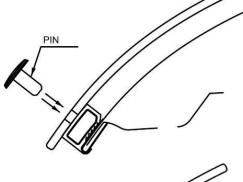
10. Insert a pin through the protector and into the clip body.
