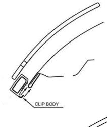
9. Place a clip body over one of the antiabrasion pads on the edge of the hood.
