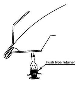
4. Insert 3 of the "push-type retainers" through the hole in the metal bracket, and into the hood.
