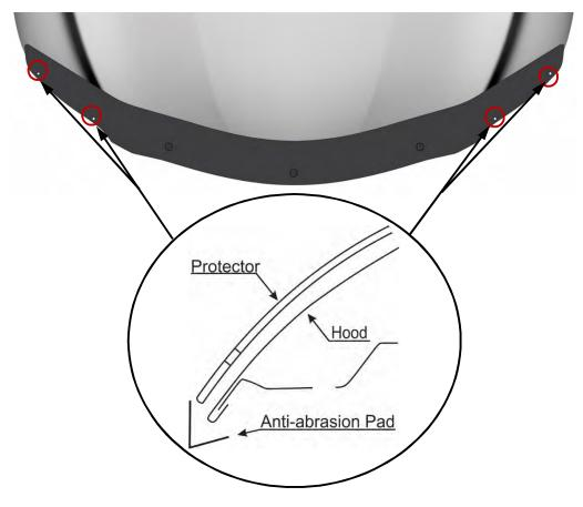
8. Peel and fold the remaining 4 antiabrasion pads in half over the edge of the hood in line with the two holes in the protector over each of the headlights.
