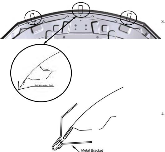
3. Open the hood of the vehicle. Peel and fold (3) anti-abrasion pads in half over the edge of the hood, in line with the (3) holes under the hood, as shown.
