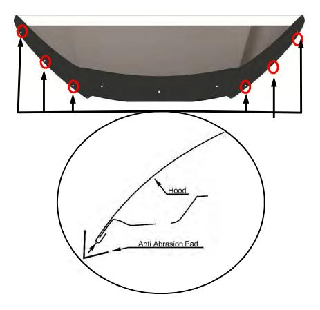
8. Peel and fold the (6) remaining anti-abrasion pads in half over the edge of the hood, in line with the three holes in the protector over each of the headlights.
