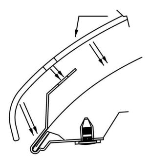
5. Insert (3) push-type retainers through the metal brackets and into the hood.
