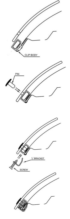
9. Place a clip body over one of the antiabrasion pads on the edge of the hood.
