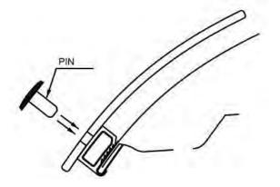
9. Insert a pin through the protector into each of the clip bodies.
