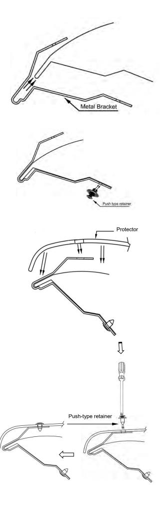
3. Install Metal Brackets over the anti-abrasion film pads installed in the previous step. Align the hole in the bottom leg of the bracket with the round hole in the hood. See Illustration.
