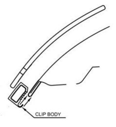
8. Place a clip body over each of the anti-abrasion pads on the edge of the hood.
