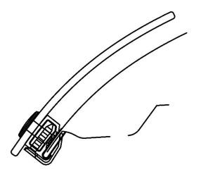
11. Make sure all the components are well seated together and the protector is centered on the hood, then tighten the screws into the clips.
