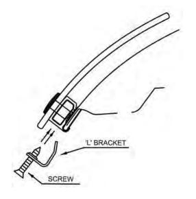
10. Insert a screw through an 'L'- bracket and into the clip body.
