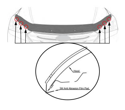
7. Peel and fold an anti-abrasion pad in half over the edge of the hood in alignment with the holes in the protector at the six locations over the headlights.
