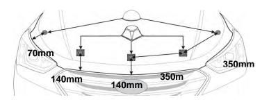
2. Open the hood of the vehicle. Peel and fold an antiabrasion film pad in half over the edge of the hood, in the locations shown.
