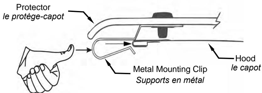
**NOTE: Ensure brackets are completely seated against the hood edge.**
