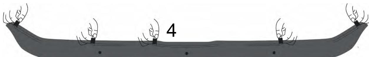
5. Install the protector by aligning the metal brackets with the abrasion pads and pushing the brackets over the hood edge until they are fully seated. Make sure tape liner tabs are accessible. **\*\*Push on the metal brackets, not the hood protector\*\***
