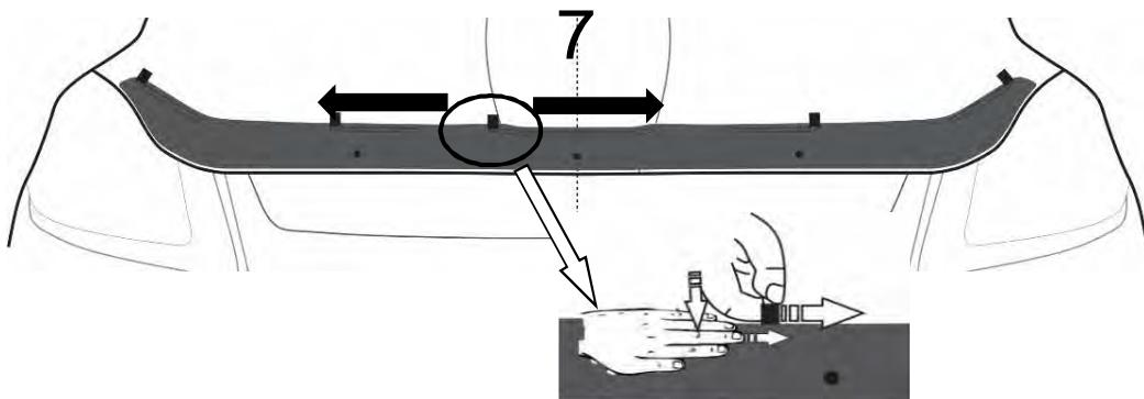
8. On some vehicles it may be necessary to adjust the hood bumpers and/or latch for proper clearance.
