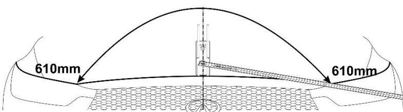
1. Assemble the installation tape measure as shown in the illustration.
