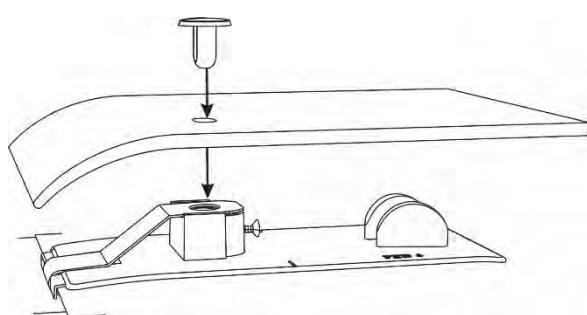
13. Peel and fold an anti-abrasion pad in half over the hood edge between the fingers on each pedestal.
