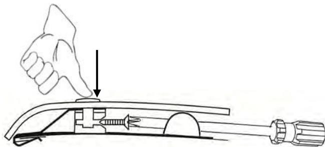
16. Starting at the center location, tighten all the screws that were loosely installed in step 15. To ensure proper seating of the components, maintain slight pressure on the pin while simultaneously tightening the screw. **Repeat for all remaining pedestal locations.**
