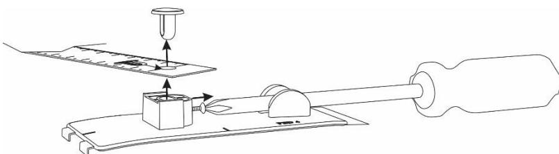
3. Assemble the installation tape measure as shown in the illustration.
