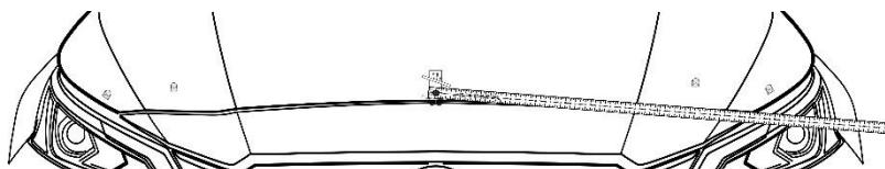
The positions of the pedestals are shown in the illustrations. Use the center mark on the leading edge of the pedestals for accurate measuring. The fingers incorporated on the leading edge of the pedestal will help ensure the correct position relative to the hood edge. When correctly positioned the fingers should contact the leading edge of the hood.
