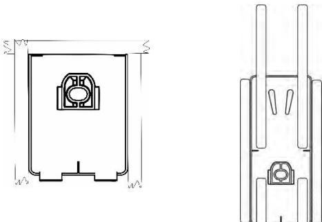
5. Using the repositionable tape strips, temporarily attach the two (2) small adhesive pedestals at the location indicated in the illustration.
