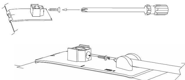
12. Start a screw into each pedestal a few turns. The tip of the screw must not protrude into the hole where the attachment pin will later install.
