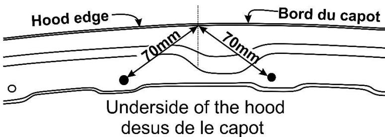
2. Find and mark hood center. Open the hood and using the method illustrated, find and mark the center of the hood at the edge.
