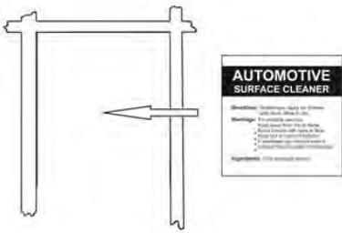
10. Remove the pedestals and thoroughly clean the outlined area with the alcohol wiping pad. Wipe dry with a clean cloth or paper towel. This will insure all wax, finger prints and oils are removed from the hood surface in the bonding area.
