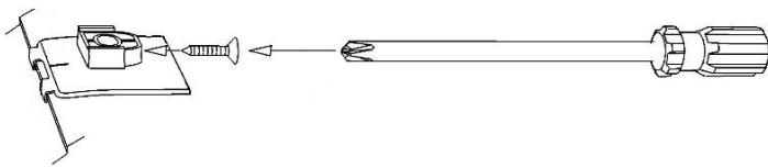
10. Lower hood and start a screw into each pedestal a few turns. The tip of the screw must not protrude into the hole where the attachment pin will install later.
