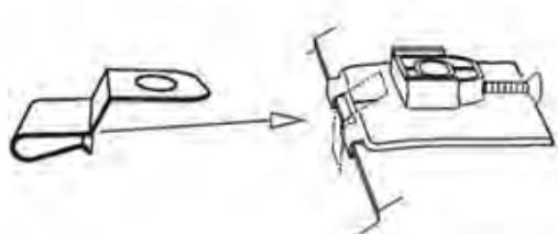
12. Push a type C metal mounting bracket over the hood edge. Align the hole in the bracket with the hole in the pedestal.
