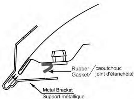
9. Loosely install truss head screws through the metal brackets and into the expansion plugs, making sure the brackets are well seated against the edge of the hood. See *Illustration*.
