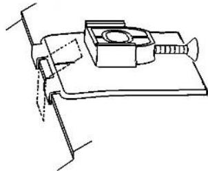
11. Peel and fold a small anti-abrasion pad in half over the hood edge between the fingers on each pedestal.
