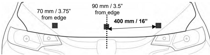
1. Install the (3) Bumpers as shown. **Bumpers must be installed on the hood, not on the protector.** If the Bumpers are installed on the protector, they may wear through the paint.
