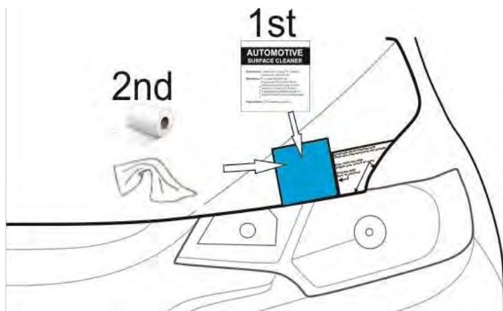
3. Using the automotive surface cleaner, thoroughly wipe the shaded area of hood surface shown in the illustration followed by drying with a soft cloth or paper towel. This will insure all wax, finger prints and oils are removed from the hood surface in the bonding area.
