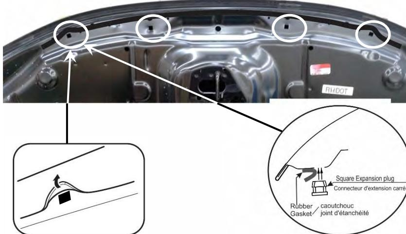
6. Open the hood of the vehicle. Fold back the rubber gasket from the locations shown in the illustration, exposing the (4) square holes. Install (1) expansion plug into each hole.
