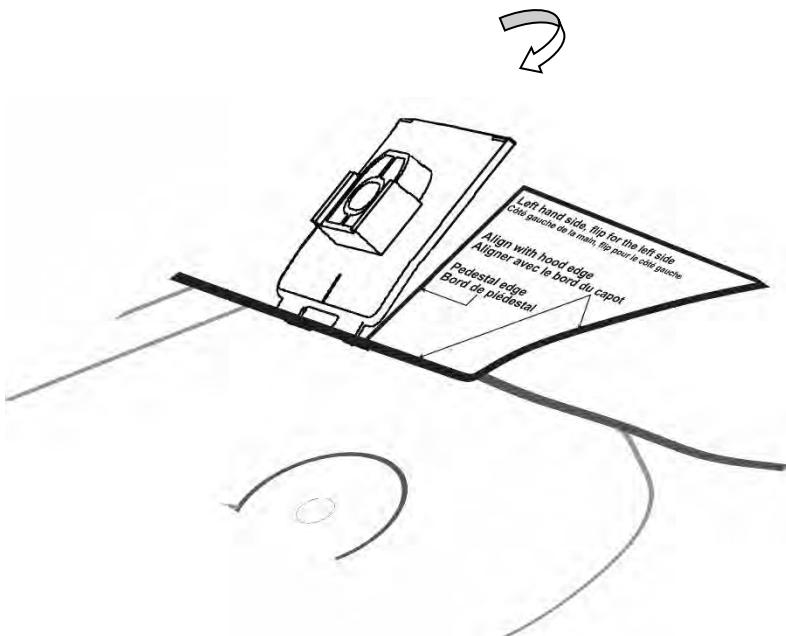
4. Remove the protective backing from the pedestal, align with edge of template and install on the hood surface. **Use caution to avoid contaminating adhesive surface.**
