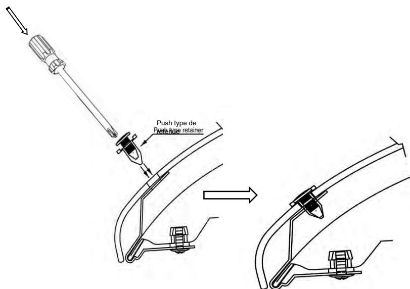
13. Place the protector on the metal brackets. Align the 4 center most holes in the protector with the holes in the metal brackets. Install a "push type retainer" through the hole in the protector, and into the bracket. Ensure the protector is seated against the metal bracket and push the center pin of the retainer assembly to lock it into place. Repeat for 3 remaining positions.
